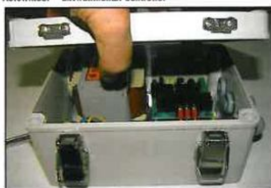
Power box accepts open/close signal from your controller & supplies Autowinder with 24v DC current
